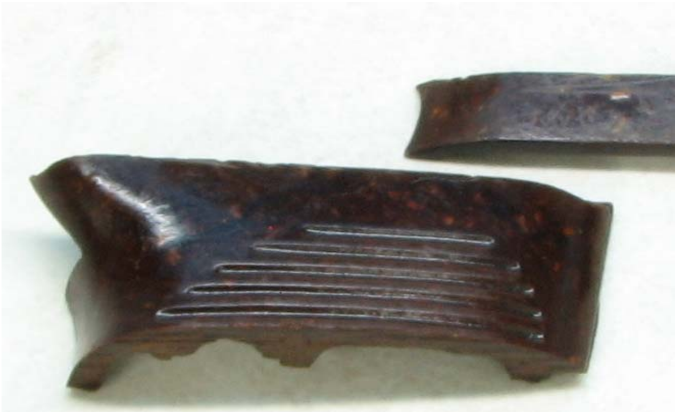
Figure 1a (above) and 1b (below) – Section 1 (CLP immersed) with section 0 (control section) in background at time +1 year.
