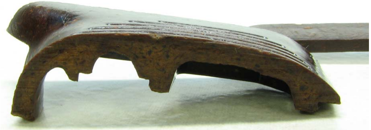
Figure 1a (above) and 1b (below) – Section 1 (CLP immersed) with section 0 (control section) in background at time +1 year.
